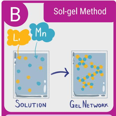
A slowly heated solution leads to a network of cathode material with good homogeneity (regular, repeating order).
