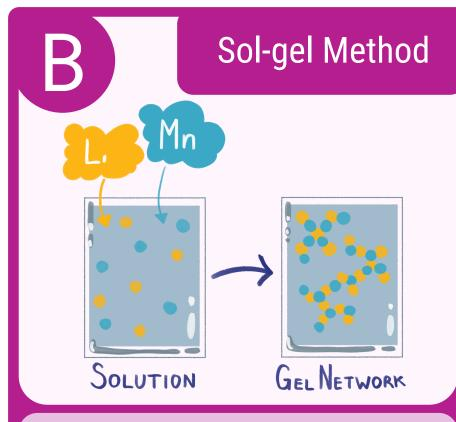
A slowly heated solution leads to a network of cathode material with good homogeneity (regular, repeating order).
