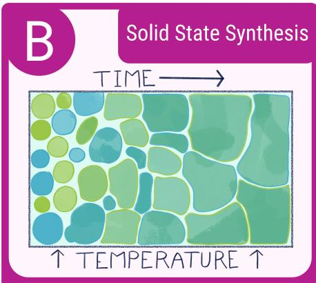
The materials are ground together and heated at high temperatures. It can produce more crystalline structures, so the material is more ordered by forming more regular crystals.
