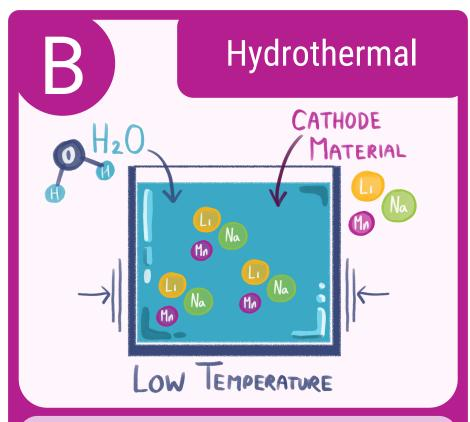
Materials are manufactured using water, as a solvent, at low temperatures. Sometimes, pressure is used to create interesting particle morphology.
